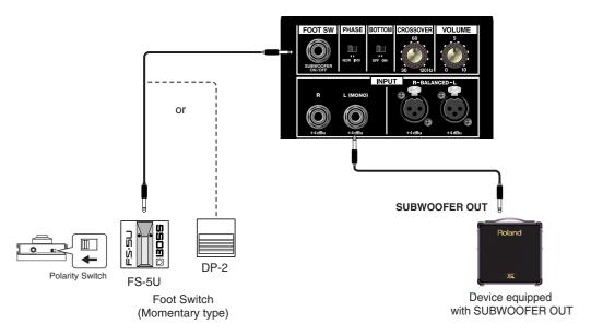
Use a 1/4" phone audio cable to connect the SUBWOOFER OUT on the device featuring the SUBWOOFER OUT connector to the KCW-1's INPUT L (MONO).
