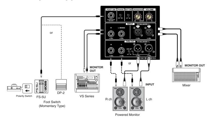
Input signals from the VS Series and other output devices to the INPUT connectors. Connect DS Series powered monitors or similar devices to the KCW-1's THRU OUT.
