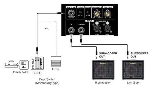
Use 1/4" phone audio cables to connect both the R (Master) and L (Sub) SUBWOOFER OUTs on the KC-550/350 or other devices to the KCW-1's INPUT L and R.
