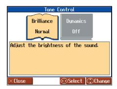
**5.** Press the cursor up or down button to change the brightness setting.
