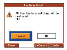
**2.** Press the cursor right button to select <OK>, then press the [O] button; the Factory Reset is executed.
