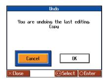
Selecting <Cancel> with the  $\bigcirc$  cursor button and pressing the < O > button returns the "Song Edit" screen to the display, and the undo of the edit is cancelled. If you select <OK> and press the < O > button, the editing operation indicated in the screen is undone.
