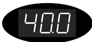
The last three digits are indicated in the display. "440.0 Hz" is indicated in the figure above.
