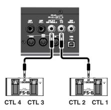
\* The following shows the correspondence between the foot switch and CTL function when two foot switches are connected using a special connection cable (Roland PCS-31: sold separately).
