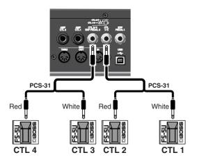
\* When connecting foot switches individually, the settings for the CTL Function 1 and CTL Function 2 are enabled.
