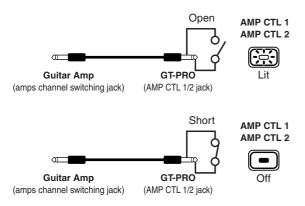
\* To determine how the amp channels are switched when the circuit is open and shorted, refer to the amp owner's manual, or actually confirm the sounds by operating the amp.
