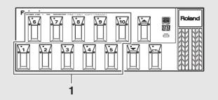
**1.** Select the number of the patch you want to switch to by pressing the corresponding number pedal.
