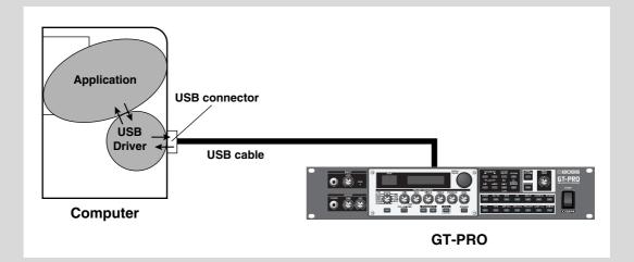
The explanation about installing and setup the driver is organized according to the computer and driver mode that you are using. Please proceed to the following pages.
