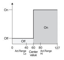
\* When using a foot switch or other on/off switching controller as the source, leave these at "Lo: 0" and "Hi: 127." With certain settings, the value may not change.
