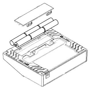
When the batteries run down, the POWER indicator gets dim. If this happens, replace with new batteries.
