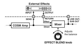
The knob settings can be adjusted to accommodate for both series and parallel connections.
