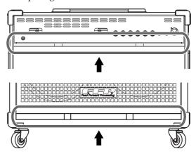
Do not allow the cooling vents on either side of the unit to become blocked. Obstructing the vents may result in damage or other problems.
