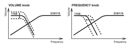
The aim of these adjustments is to achieve a smooth, continuous link in the low frequencies between the 210/115 and the 115X.
