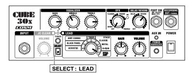
DYNA AMP is an original amp that uses relative picking strength to create changes in distortion depth.
