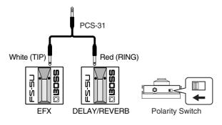
When you connect only one foot switch by mono cable, you can only use it to turn EFX on and off.
