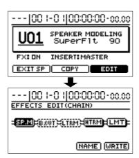
3. Use [CURSOR] to select the various speaker modeling blocks, and rotate the TIME/VALUE dial to turn a particular block on or off.
