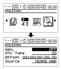
4. To enable synchronization using MTC or MIDI clock, use [CURSOR] and the TIME/VALUE dial to set the following parameters.
