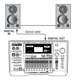
When connecting monitor speakers other than the DS-90A/DS-50A, connect as shown below.
