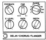
Modulation function will not work by setting the DEPTH knob too low. This setting will produce the Delay effect only.
