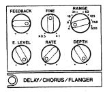
The DEPTH knob is set at the maximum. Then when the FEEDBACK knob is rotated clockwise, the flanging effect is obtained.
