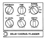
The chorus effect will be obtained by rotating the DEPTH knob clockwise. The FEEDBACK knob should be set at the minimum.
