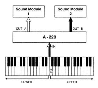
Setup: Connect sound module 1 to MIDI OUT A, and sound module 2 to MIDI OUT B.
