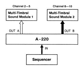
Setup: Connect sound module 1 to MIDI OUT A, and sound module 2 to MIDI OUT B.
