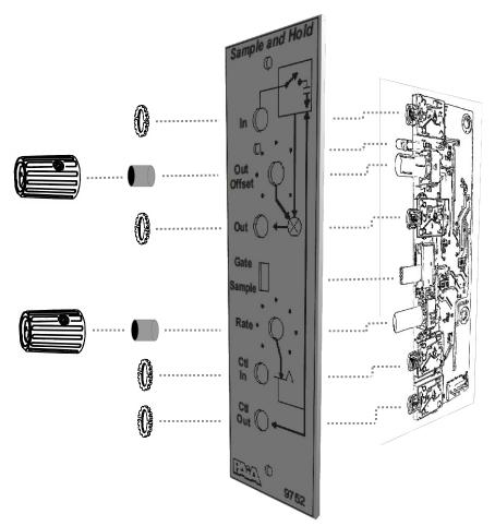
Fig. 1A Attach board to panel using connector nuts, shim control shafts, and rotate controls to minimum and tighten set-screw knobs to agree.
