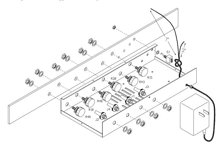
Fig 6. The only hardware that attaches the case to the rack panel is the threaded bushings of the pots and power switch. Wiring which is already connected when the Case and Panel are joined is not shown for clarity.
