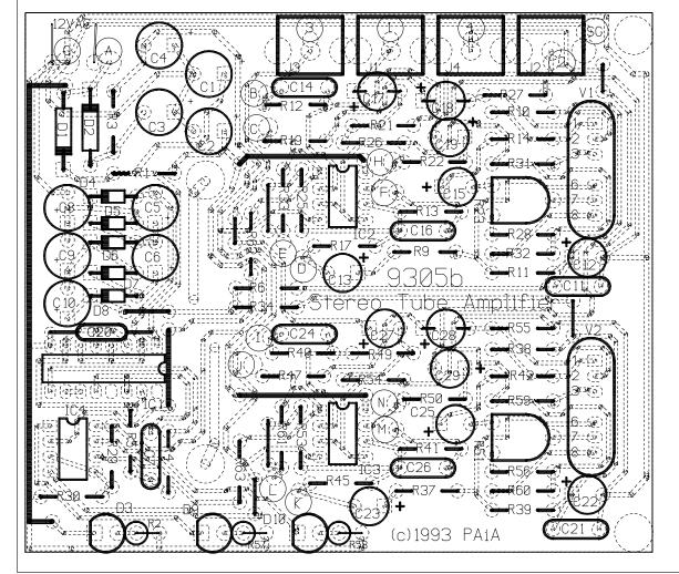
Fig 1.This view of the circuit board with phantom traces will be useful if you need to trace out the circuit.
