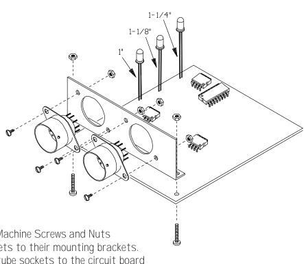
Fig 3. Four #4 X 1/4" Machine Screws and Nuts attach the tube sockets to their mounting brackets. After wires from the tube sockets to the circuit board are in place, the bracket is temorarily screwed to the circuit board with the same #4 X 1/2" screws and nuts which will later hold the assembly in the case.
