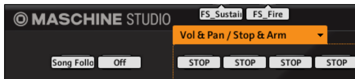
Footswitch inputs of the MASCHINE STUDIO controller
