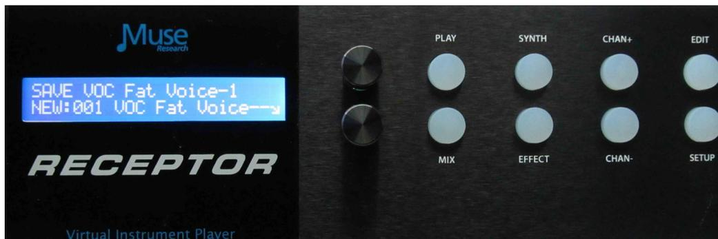
Simply use the bottom knob to select the location you want to save, and then press the bottom encoder to either create (if "new") or save (if writing over) the preset. Writing a preset takes a moment, after which time it will say "Created" on the display. All naming is automatic, but if you want to give them specific names you can do so using the Graphical User Interface.
