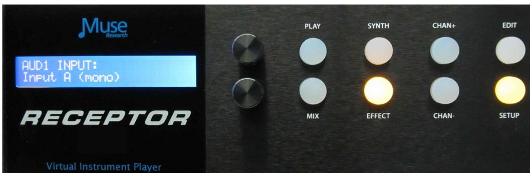
3. Turn the gain control to minimum on Input A and plug in your acoustic guitar. Turn the bottom encoder to select "TAG FX Acous Gtr" and then turn the top knob to select the preset "007 AcstcGuitar" Press the encoder button to load the patch. Of course if there is a different preset you'd like to use on the guitar, feel free to select it now.
