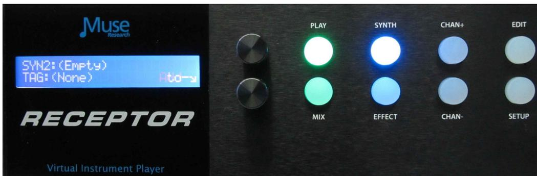
4. Select the TAG and preset of interest, say "Airy Pad" from the "TAG:Synth Pads" category. Press the knob to load this preset. Now press the "PLAY" button to hear both sounds combined together. What we've done is layered the Electric Piano and the Pad sounds together, which creates an entirely new sound. You can adjust the volume of either sound by pressing MIX and selecting the channel of interest to adjust the Electric Piano or Pad volume levels respectively.
