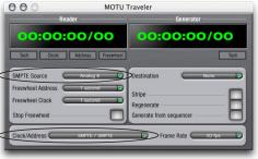
Launch the MOTU SMPTE Console to specify the time code input, frame rate and amount of freewheel. Also, confirm that the *Clock Source/Address* is *SMPTE/SMPTE*. For details about the other settings, see chapter 12, "FireWire SMPTE Console" (page 87).
