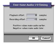
Figure 8-2: Fine-tuning the timing of audio playback and recording.
