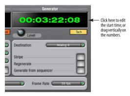
Figure 12-2: Setting the time code start time.
