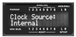
Figure 6-2: In setup mode, the LCD displays a setup parameter in the top row of the LCD and the current setting in the bottom row.
