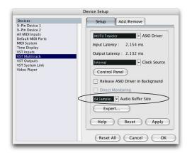
Figure 10-4: In Cubase SX or Nuendo, choose Devices menu> Device Setup and click VST Multitrack to access the window above and the Audio Buffer Size setting.
