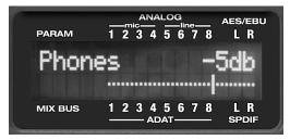
Figure 6-3: For many settings, the LCD "zooms in" on the setting as you adjust it.
