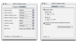
Figure 8-1: Choose Setup menu> Configure Audio System> Configure Hardware Driver to open the dialog shown above and access the Traveler Core Audio driver. To access the rest of the Traveler settings, open the MOTU FireWire Audio Console.
