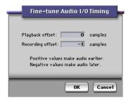
Figure 7-2: Fine-tuning the timing of audio playback and recording.
