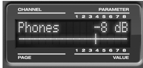
Figure 6-9: The LCD provides feedback as you adjust volume.
