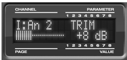
Figure 3-6: Setting the input trim for a TRS analog input.
