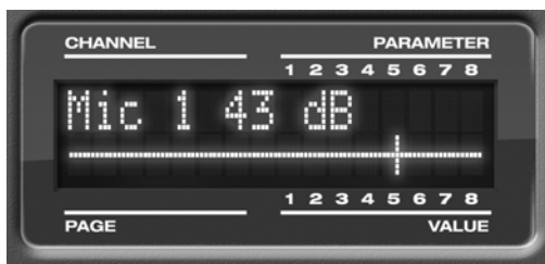
Figure 3-3: The LCD gives you feedback as you turn the TRIM knobs for the four mic/guitar inputs.
