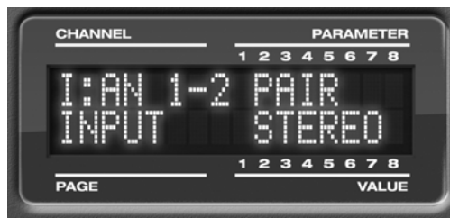
Figure 3-5: The settings for analog inputs 1 and 2 (as a pair).
