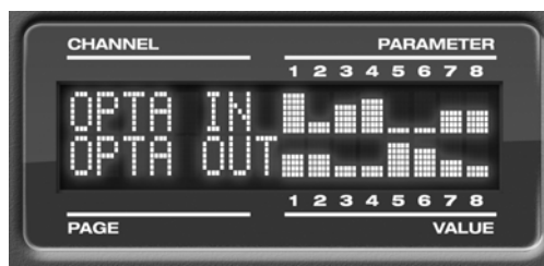
Figure 6-4: Multi-channel metering in the LCD.
