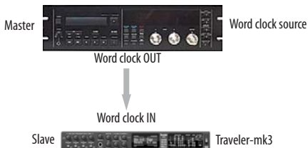
Figure 3-20: Slaving the Traveler-mk3 to word clock. For the Traveler-mk3 clock source, choose 'Word Clock In'.
