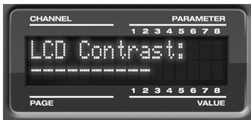
Figure 6-11: In setup mode, the LCD displays a setup parameter in the top row of the LCD and the current setting in the bottom row.
