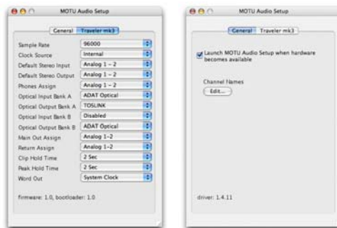
Figure 7-1: Choose Setup menu > Configure Audio System > Configure Hardware Driver to open the dialog shown above and access the Traveler-mk3 CoreAudio driver. To access the rest of the Traveler-mk3 settings, open MOTU Audio Setup.
