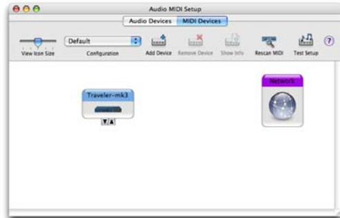
Figure 4-1: The Traveler-mk3 interface as it appears in the MIDI tab of Audio MIDI Setup.
