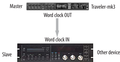
Figure 3-19: Slaving another digital audio device to the Traveler-mk3 via word clock. For the Traveler-mk3 clock source, choose any source besides word clock, as it is not advisable to chain word clock.
