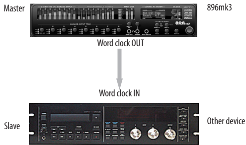
Figure 4-18: Slaving another digital audio device to the 896mk3 via word clock. For the 896mk3 clock source, choose any source besides word clock, as it is not advisable to chain word clock.
