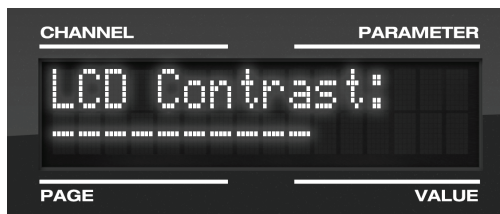
Figure 6-8: In setup mode, the LCD displays a setup parameter in the top row of the LCD and the current setting in the bottom row.
