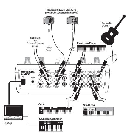
This diagram shows an acoustic guitar connected to channel 1, plus a stereo performance synth like a Nord Lead on channel 2, a good organ like a Korg CX-3 on channel 3, and an electronic piano on channel 4 (with a dab of chanel #5 behind each ear for good measure).
