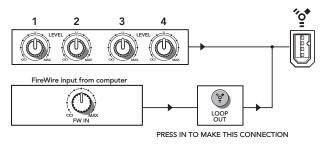
The mains and phones outputs are not affected by the switch, and always provide a full mix of channels 1 to 4 and the 2-channel FireWire input.
