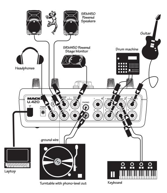
This diagram shows a guitar connected to channel 1, plus a stereo synth and drum machine connected to channels 2 & 3. A turntable is connected to the phono inputs on channel 4. Use the left aux send to connect to a Mackie SRM450 for stage monitoring. The U.420 will automatically sum the stereo signal to mono if you use the left aux output only.
