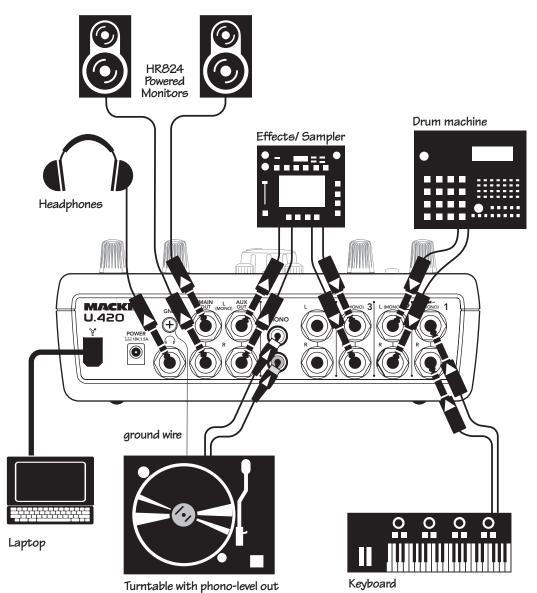
This diagram shows a stereo synth, and a drum machine connected to channels 1 & 2, and a turntable connected to the phono inputs of channel 4. The stereo aux output sends signals to the effects/sampler, and the wet signal is returned into channel 3.
