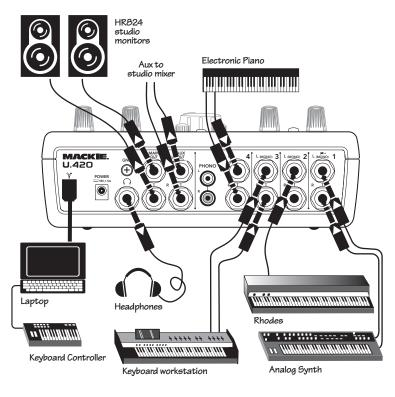
This diagram shows a stereo keyboard workstation, a groovy analog synth, an electronic piano, and an electric organ connected to channels 1–4.
