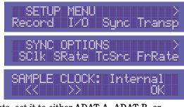
connected to one of the digital optical inputs, set it to either ADAT A, ADAT B, or ADAT C, depending on which digital port the master device is connected to.
