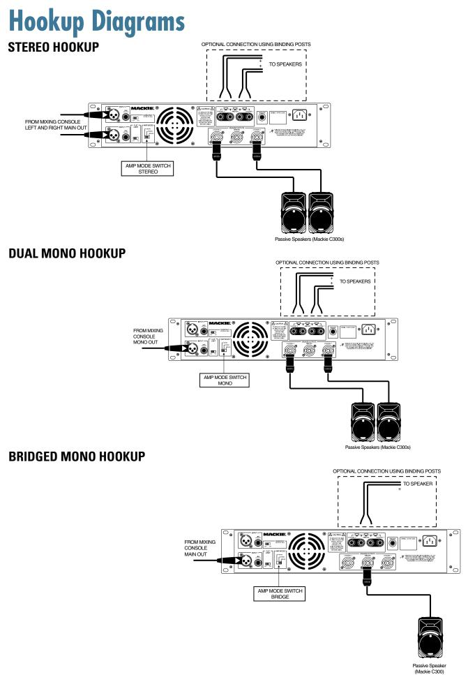
STEREO, DUAL MONO, AND BRIDGED MONO
