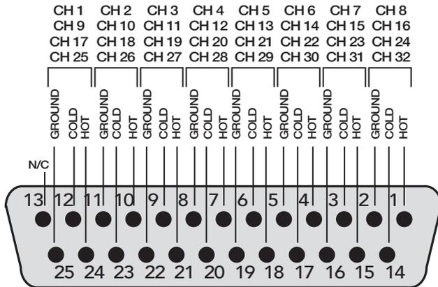
Several companies make DB25-to-DB25 cables specifically for audio, with proper shielding to reduce crosstalk and noise.
