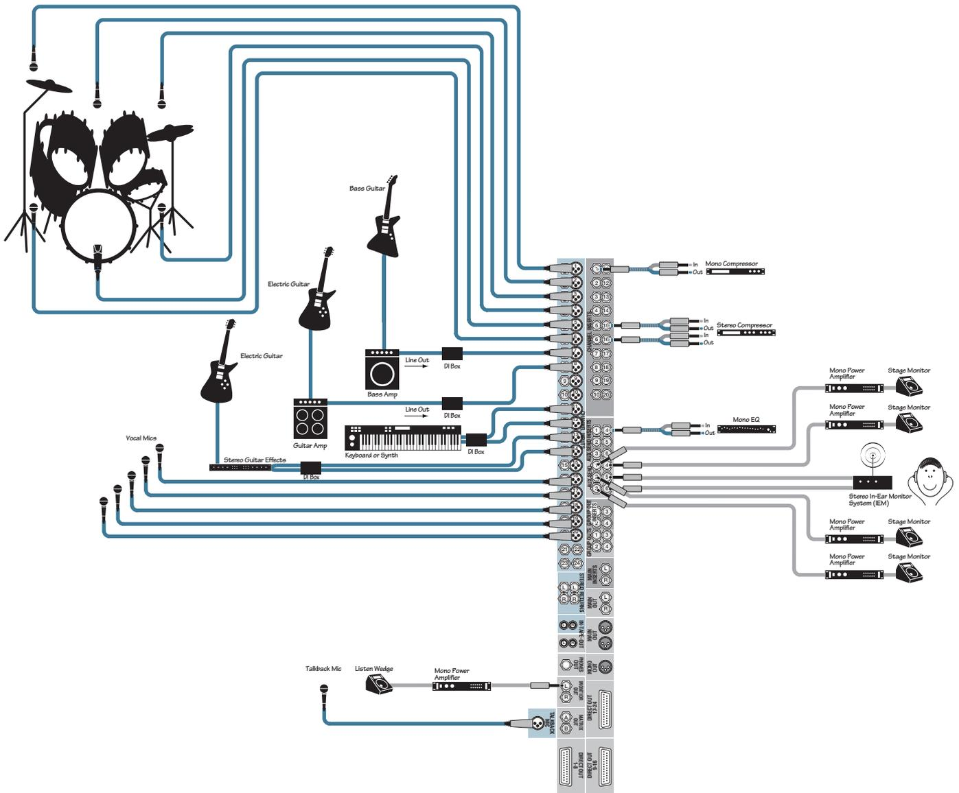
*This drawing shows the flexibility of the Onyx 4•Bus for creating different monitor mixes. Auxes 1-4 provide separate monitor mixes for four floor wedges. Auxes 5-6 provide a stereo monitor mix for an in-ear monitor (IEM). The Aux Inserts can be used for in-line graphic EQ for each monitor send. A listen wedge is connected to the Monitor Out, allowing you to solo and listen to each monitor mix. The Talkback Mic lets you talk to the talent through the monitors (Aux Sends).*
