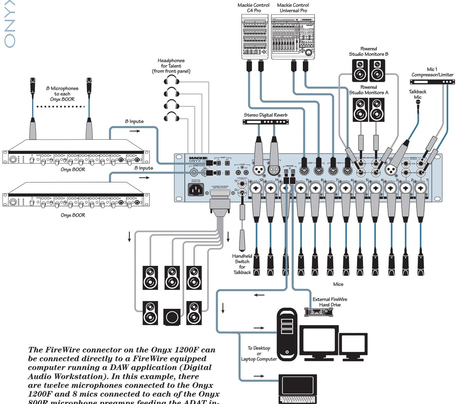
*The FireWire connector on the Onyx 1200F can be connected directly to a FireWire equipped computer running a DAW application (Digital Audio Workstation). In this example, there are twelve microphones connected to the Onyx 1200F and 8 mics connected to each of the Onyx 800R microphone preamps feeding the ADAT inputs on the Onyx 1200F, for a total of 28 microphone feeds to the DAW.*
