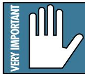
**Never plug single-ended (unbalanced) microphones or instruments into the MIC input jacks if the PHANTOM power is on.**
