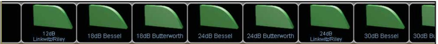
Note: The Linkwitz-Riley filter is only available in 12 dB, 24 dB, 36 dB, and 48 dB versions. The 12 dB and 36 dB Linkwitz-Riley crossovers require a polarity inversion between adjacent crossover pairs in order to maintain a constant magnitude characteristic. For example, when using a 2-way 36 dB Linkwitz-Riley crossover, invert the polarity of the high output channel. When using a multi-way crossover, invert the polarity of every other output channel.
