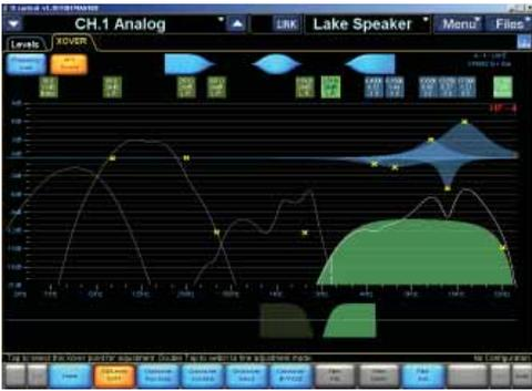
Here is a more complex system, a tri-amped EAW KF695z with a subwoofer.
