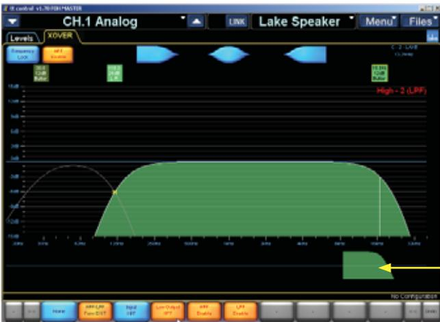
Click and drag left and right on the HPF icon in the bottom of the window to change the cutoff frequency of the filter.
