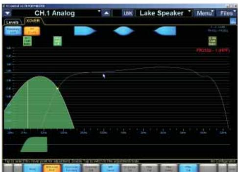
Here is the low end of the EAW system, which your EAW 250z subwoofer would receive.
