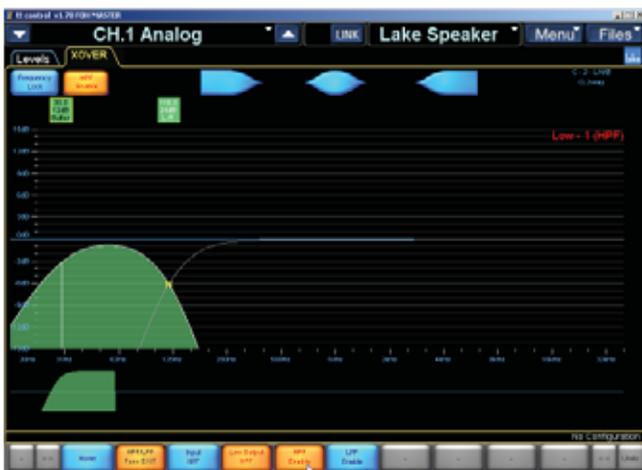
Click the HPF Enable button to insert a high-pass filter into the low-frequency output. Click and drag left and right on the LPF icon in the bottom of the window to change the cutoff frequency of the filter.
