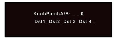
This page displays the current Soft knob parameter value, as well as the *Effect* parameters which are patched to it.
