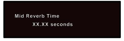
Pressing the front panel VALUE key will display all of the current parameter values for the selected page. in this example, pressing VALUE will cause the following display to appear:
