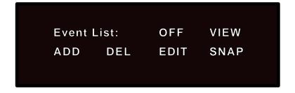
This page allows creation and modification of a list of up to 50 events triggered standard timecode or MIDI timecode. Four main functions are provided: Add, Delete, Edit and Snap. (For more information, see Chapter 6: Time Code Operation.
