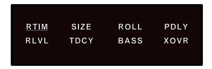
The buttons directly above and below each display entry will select that parameter. Once selected, parameters can be adjusted over their entire range with the Soft knob. The parameter and its current value will appear on the display as long as the Soft knob is being adjusted. In the example above, "RTIM" has been selected — turning the Soft knob will alter the parameter value, and cause the display to show:
