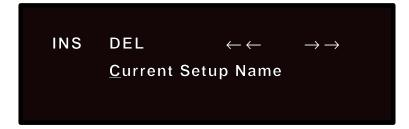
The bottom line of the display shows the name of the current setup, with a cursor positioned under the first character. The two keys directly above the left and right arrows cause the cursor to move left and right to select other characters.
