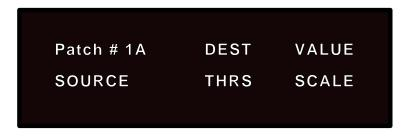
**Destination**: This is used to select the effect parameter that the MIDI controller is patched to. The available parameters are based on the algorithm that you are currently running.
