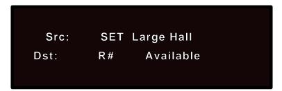
The top line of the display shows the source (Src) — the currently selected setup name. The bottom line shows the destination (Dst) — the register number into which the setup will be copied. Use the Soft knob to select the register number you want, then press STORE again. The display will return to the last Setup Edit page.
