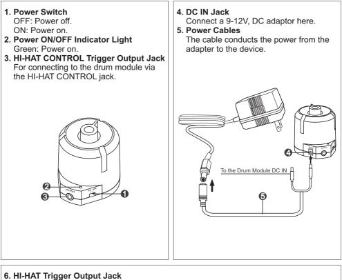
For connecting to the drum module via the HI-HAT INPUT jack.
