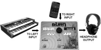
In case the input signal level is too weak or it is too hot to overload the DSP and needs to be reduced, it is possible to compensate the difference between the input and the output level by adjusting the value of the page [I/O] OUT BOOST up to a maximum of 195%, which corresponds to nearly +3 dB (loudness almost doubled). This function works only when the page [I/O] RIGHT IN is set on OFF.
