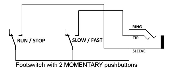
PLEASE NOTE: when using this kind of footswitch, you must set the option [MIDI] SPEED TYP to LATCHED because the accessory uses momentary switches, and the latching must be made by the software.
