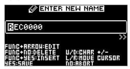
The [LEFT] and [RIGHT] arrow keys are used to navigate between the characters. Turning the *LEVEL/DATA* knob or pressing the [UP] or [DOWN] arrow keys selects the characters. [FUNC] + [NO] will erase letters. Press and hold [FUNC] to access the pop-up naming menu.
