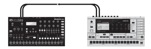
Thanks to the neighbor routing, all the filters of the Analog Four can be used for providing an immense mono filter bank consisting of 8 filters plus 4 overdrive circuits. The setup can be either serial or parallel. It can, of course, be set up for stereo filtering as well. In this scenario, 4 filters are available for the left and right channels.
