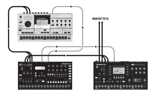
The Analog Four thrives with other Elektron gear. In this example, it is used with an Octatrack and a Machinedrum. The Machinedrum main output is connected to the Analog Four inputs. The Analog Four main output is connected to one of the input pairs of the Octatrack. The main outputs of the Octatrack go to the PA. The Machinedrum and Analog Four are MIDI slaved to the Octatrack.
