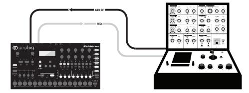
The CV/Gate outputs and the external inputs allow an external oscillator to be used with the internal Analog Four oscillators. Use this trick when you want a different (perhaps old, quirky and unpredictable yet charming) oscillator to provide the fundamental tone but still want the control and modulation power of the Analog Four.
