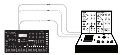
The CV/Gate track of the Analog Four is made for controlling external, CV/Gate equipped, analog gear. In this scenario, a vintage analog synthesizer is controlled by the Analog Four. The pitch and filter cutoff will be controlled.
