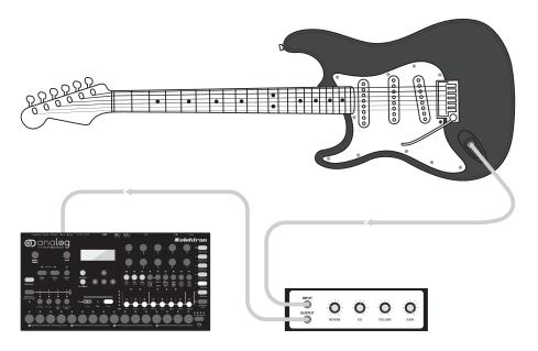
In this setup example, the Analog Four is used for processing the sound output from an electric guitar. The first, most basic method uses the FX track to turn the Analog Four into an effects box sporting the Wideshift Chorus, Saturator Delay, and Supervoid Reverb effects. The second, more elaborate method routes the sound through Track 1 and allows all the sound-shaping possibilities offered by the FILTERS, AMP, ENV and LFO.
