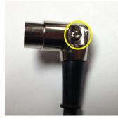
Loosen the screw on the side of the headshell. It is not necessary to remove the screw.
