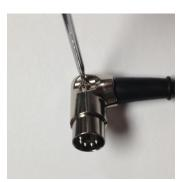
Tighten the screw on the side of the headshell.
