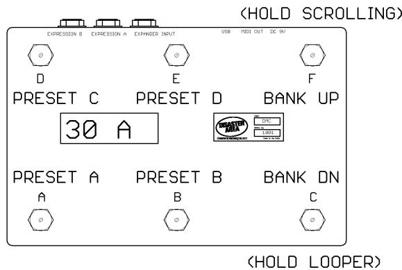
Pressing the button for the currently selected preset bypasses all connected devices. Pressing the current preset also sends MIDI program change 0 on the fourth MIDI channel.
