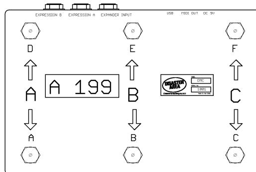
"A" device - Buttons A and D step up and down through patches on MIDI Channel 1 (Timeline)
