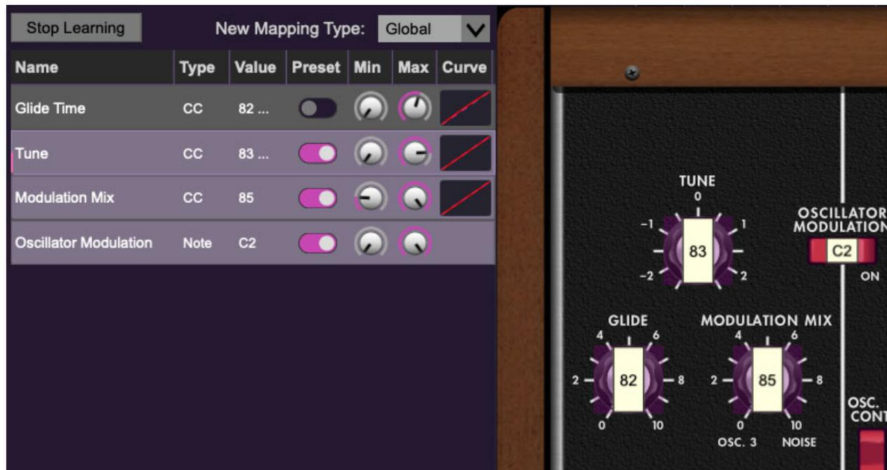
When in MIDI learn mode, any previously assigned controller numbers will show in squares. These indicate the MIDI continuous controller number of the assigned hardware control (these are also displayed in the *MIDI* library tab at left).
