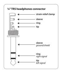
Fig. 6.6: Stereo plug for headphones connection
