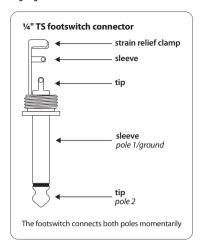
Fig. 6.1: Foot switch connector
