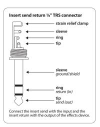
Fig. 6.5: Insert send/return stereo plug
