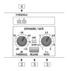
Fig. 2.2: Control elements of expander/gate section
