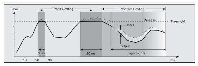
Fig. 4.3: IGC characteristic of the limiter section
