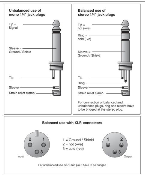
Fig. 7.2: Different plug types
