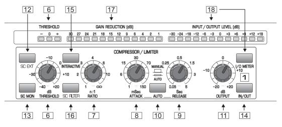
Fig. 2.3: Control elements of the compressor section
