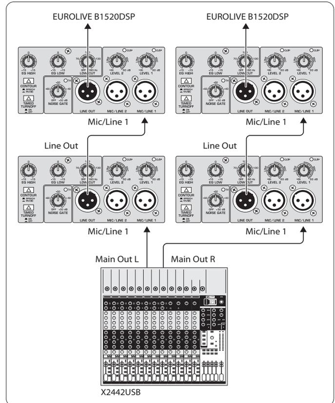
Fig. 4.3: Linking several B1520DSP speakers
