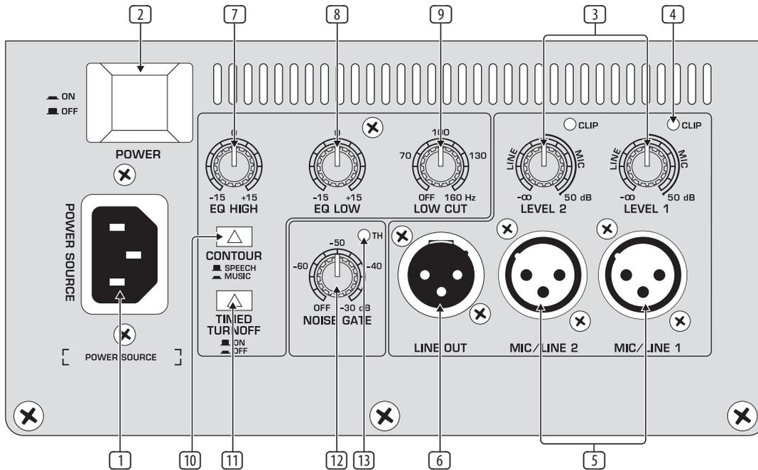
Fig. 2.1: Control elements and connections
