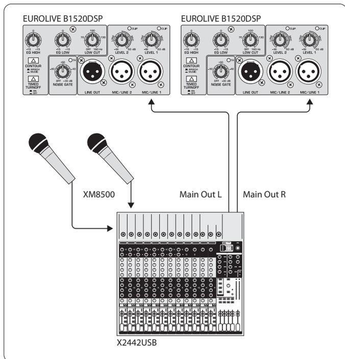
Fig. 4.2: Connecting a mixing console
