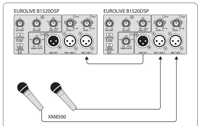
Fig. 4.1: Connecting microphones
