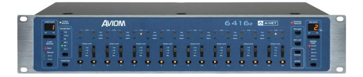
Version 2 of the 64160 Output Module provides 16 balanced mic- or line-level XLR analog outputs from a Pro64® A-Net® network. Each channel includes a four-position output level switch (mic-level and +4, +18, or +24dBu line-level), as well as three-segment level metering. Alternate analog audio outputs are provided via DB25 multipin connectors on the rear panel. The 64160 v.2 is ideally suited for applications requiring hotter analog outputs such as connecting directly to power amplifiers.
