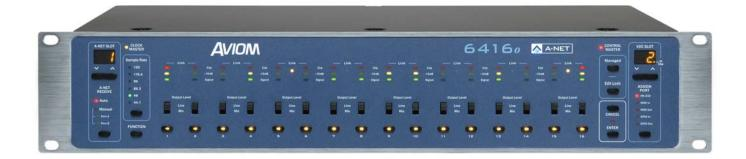
The 64160 Output Module provides 16 balanced mic- or line-level analog outputs from a Pro64® A-Net® network. Each channel includes a two-position output level switch (mic or line) and three-segment level metering. Alternate analog audio outputs are provided via DB25 multipin connectors on the rear panel.
