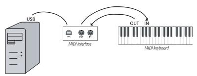
If you want to connect just, say, a sound module, rather than a keyboard, simply connect the MIDI interface's "Out" to the sound module's "In."
