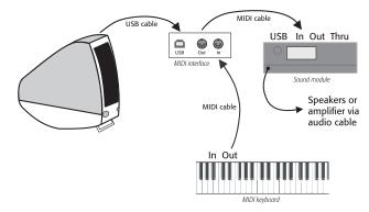
The second MIDI cable goes from the "Out" socket on the keyboard to the "In" socket on the MIDI interface.
