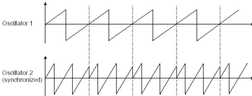
In the above image, oscillator2 is synchronized with the first and tuned to with double the tonality. The resulting waveform is unique in that it cannot be created by standard synthesis techniques such as layering or filtering.
