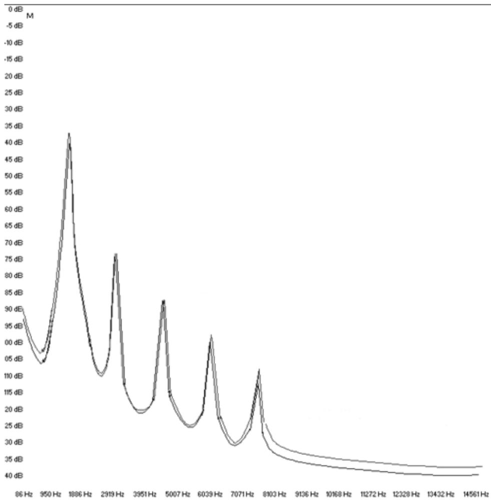
*Comparison of Harmonics generated by the filter circuits of the Prophet-V2 and Prophet 5 when in self oscillation*
