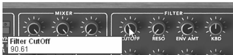
*Lower the filter cut-off frequency*
