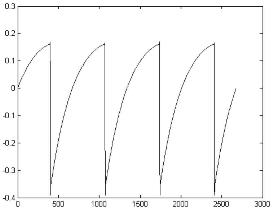
*Temporal representation of a Prophet-V2 “saw tooth” waveform reproduced by TAE*
