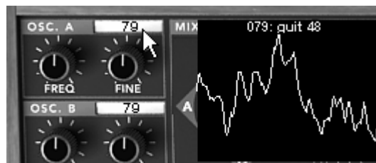
Screen for choosing the waveforms of the oscillators
