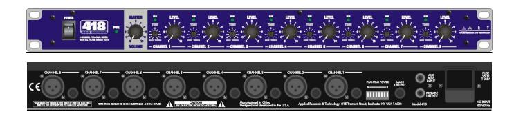
The ART Model 418 Eight Channel Personal Mixer provides eight channels of basic mic/line mixing capability in a convenient, easy-to-use rack format. The unit features a selection of XLR mic and 1/4 inch unbalanced line inputs with LEVEL and TONE controls. Additionally, phantom power is also available, and is switch-selectable on each mic input. Each line input can be converted internally to a line output for that channel.
