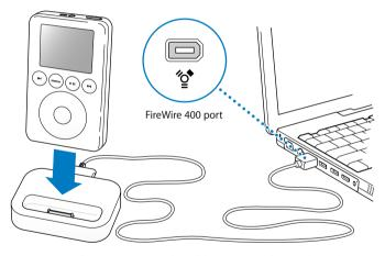
**Note:** Be sure the connectors on the cable are oriented correctly. Each connector can only be inserted one way. Your computer must be on and not in sleep mode (some models of Macintosh can charge iPod while in sleep mode).
