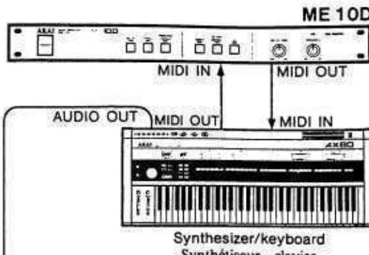
Connection procedure—refer to connection diagram I
