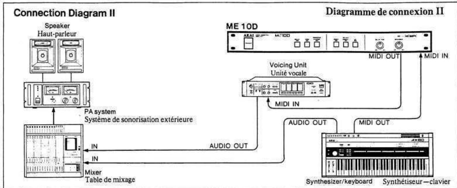
Connection procedure—refer to connection diagram II
