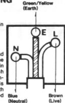
The wire which is coloured blue must be connected to the terminal which is marked with the letter N or coloured black.
